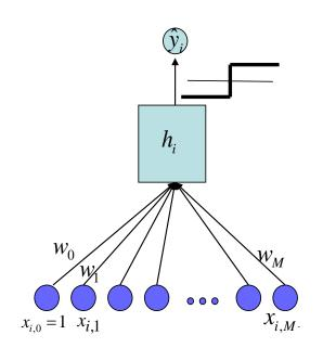
• The Perceptron calculates first a sum of weighted inputs
