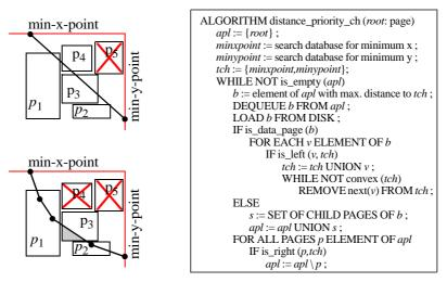
Fig. 3. The distance priority algorithm for the CH
