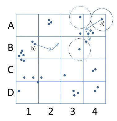
The map shown above is divided into a  $4 \times 4$  equi-grid of micro zones. 32 objects are moving on the map with initial positions as shown above. The "Area of Interest" (AoI) of an object is circular with its radius corresponding to half of the side length of a micro zone. *Note: they are shown for some objects in the Figure*.
