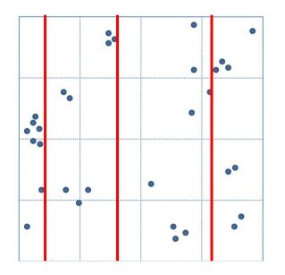
Using the sort-tile algorithm, we first need to determine how many partitions (resp. quantiles) we need per dimension:
