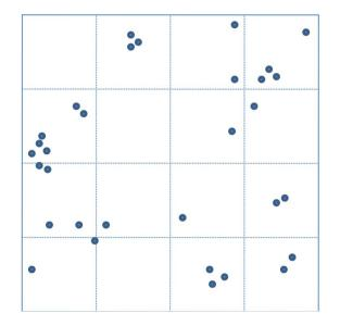
I omit drawing the tree structure here. Due to having a page size of 2, this would correspond to building a binary tree bottom up, i.e., starting with 32 objects on the leaf-node level, the next level would contain 16 nodes (since we aggregate two objects within one MBR), then the next level would have 8 nodes (again, we approximate 2 MBR objects by one larger MBR) and so on.
