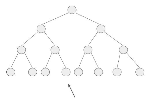
Each partition contains at most four objects  $\rightarrow$  stopping criteria is reached
