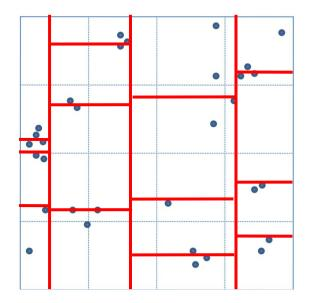
Next we need to partition along the y-axis, and due to the page limit being 2, we ensure that each partition finally contains 2 elements.
