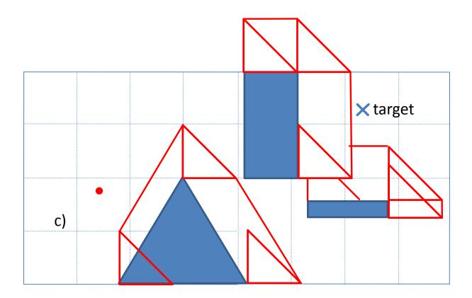
Now the shortest path to the target is again the shortest path in the visibility graph.
