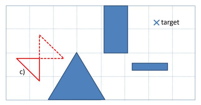
Now the shortest path to the target is again the shortest path in the visibility graph.
