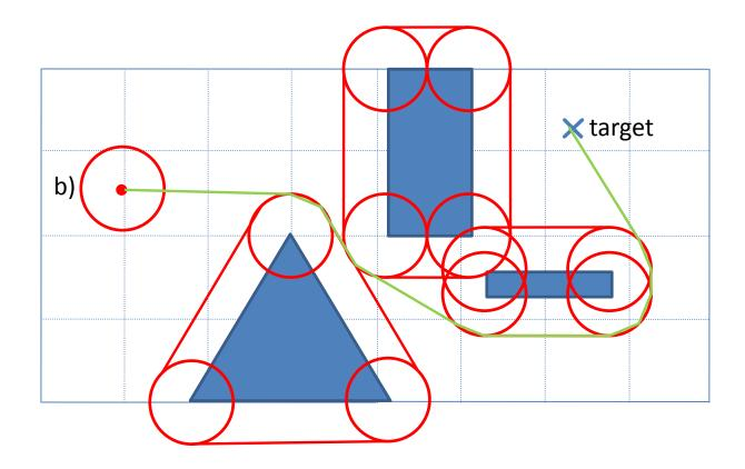
Annotation: The triangle is not invariant to point reflection-If approximated with a circle, there would be no path to the target.
