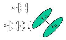
$$\Sigma_b = \frac{1}{|C|} \begin{bmatrix} \mu_1 - \overline{\mu} \\ \dots \\ \mu_m - \overline{\mu} \end{bmatrix}^T \cdot \begin{bmatrix} \mu_1 - \overline{\mu} \\ \dots \\ \mu_m - \overline{\mu} \end{bmatrix}$$
