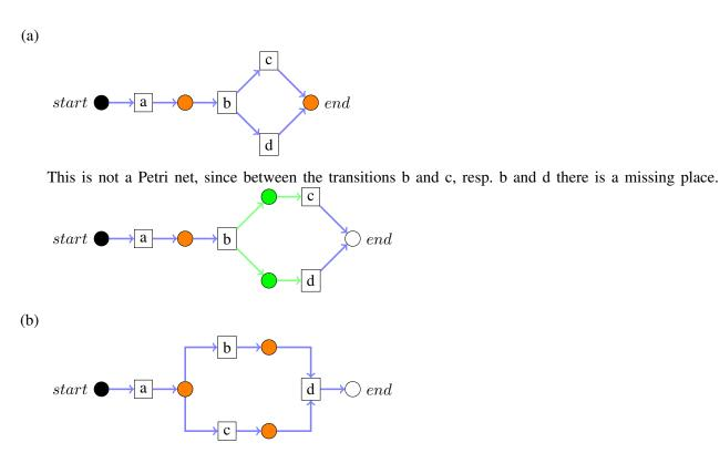
This is a Petri net and a workflow net, but it is not sound, since there are **deadlocks**. The OR-Split after the transition a gets closed by an AND-JOIN which causes a deadlock. Transition d can not fire since it will always only get one token from eighter b or c.
