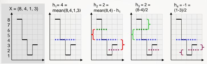
(Lossless) Reconstruction of original sequence (stream) from Haar-wavelet representation:
